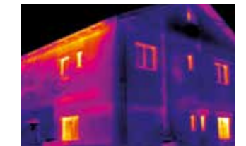
Detect energy losses from buildings: immediately identify and record thermal bridges in building fronts or shells.
