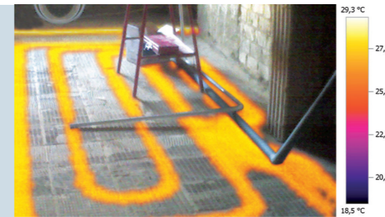
See hidden pipelines even in the real image, with TwinPix
