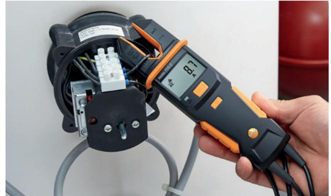
It features automatic measurement parameter recognition, exchangeable measuring tips and a voltage range up to 1000 V.
