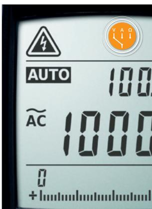
Automatic measurement parameter detection
