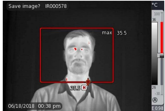
Fever Detection feature with a window on the thermal image and higher temperature marked in red
