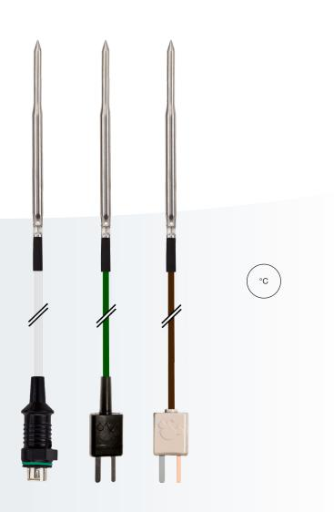
Based on the proven penetration temperature probes, customer requirements can be fulfilled even better now. For all available sensor types (NTC, Pt100, thermocouple) cable lengths up to 29.5 m can be selected in a configurator. Additionally, we introduce a more precise thermocouple probe with an accuracy of  $\pm 0.5$  °C (type T, class 1).
