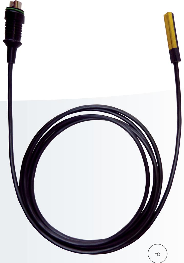
The compact, calibratable probe is suitable for temperature measurements on magnetic surfaces. The main area of application is the monitoring of processes on surfaces. The low height of 7 mm allows measurements between several layers. The temperature is recorded by the measurement contact surface of approx. 180 mm<sup>2</sup>. The magnetic area can be easily cleaned using compressed air.
