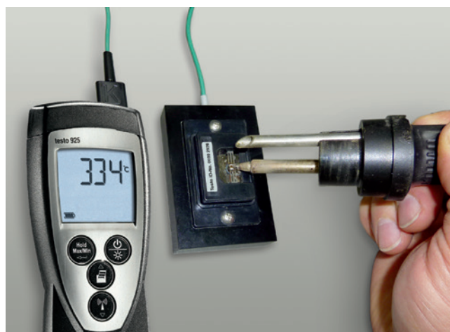
Quick and accurate verification of soldering iron temperature.
