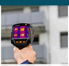
Fast detection of leaks and energy-saving potential in building management.
