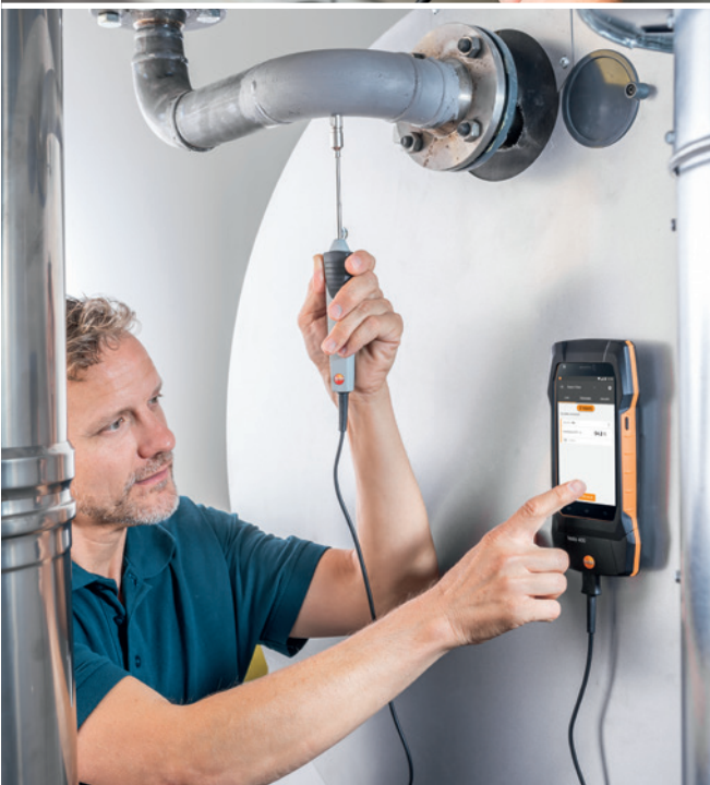
With the testo 400, you can use up to eight probes simultaneously (4 x Bluetooth, 4 x cable).
