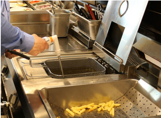
An employee tests cooking oil quality with the testo Saveris Food Stores cooking oil tester.
