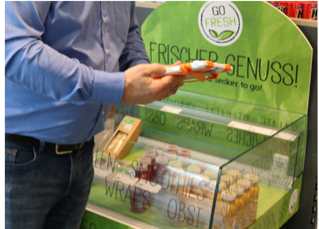
The measurement values from the online data loggers in the refrigeration units can be read out, and alarms processed, using the Control Unit.
