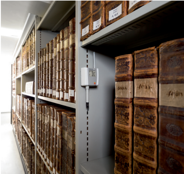
Monitoring climate in a municipal archive.
