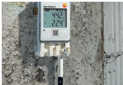
Mould prevention – building humidity (testo Saveris 2-H2 with the digital, external humidity probe 0572 2154)
