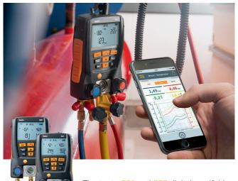
The **testo 550** and **557** digital manifolds are equipped to simplify your air conditioning system testing and servicing.
