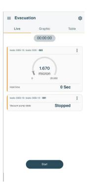
The measurement is running, the decay test has not yet started.
