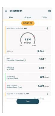
When the target values are reached, the evacuation and therefore also the pump are stopped automatically. The vacuum decay test begins. The decay test can be ended via Stop.
