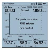
The measurement is running, the decay test has not yet started.
