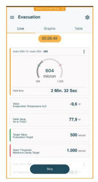
The measurement data is transferred to the testo Smart App and evaluated there.
