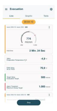
If the Auto Re-Start function has been activated, evacuation is restarted in order to restart the decay test once the decay target has been reached.
