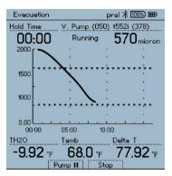
When the target values are reached, the evacuation and therefore also the pump are stopped automatically. The decay test begins.
