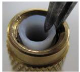
4 Put a few drops of rubbing alcohol (95%) into the sensor opening.
