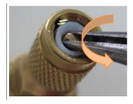
Turn a suitable screw left-handed slightly into the white seal and pull out the white seal to expose the sensor opening.
