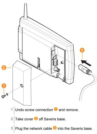
4 Connect the network cable 3 to the Ethernet.
