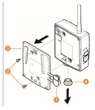
4 Unscrew and remove cover cap of cable opening 4.
