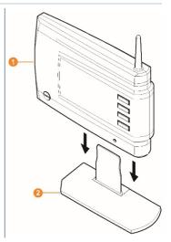
2 Set up the Saveris base at the required location.
