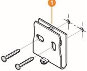
2 Using a pen, mark the locations for the fastening screws.
