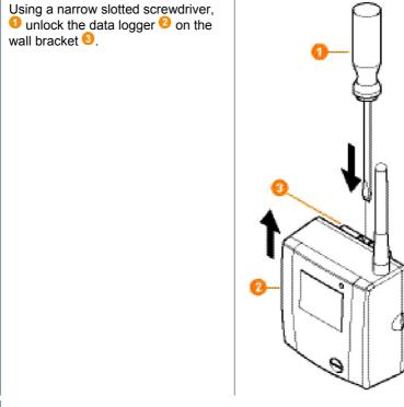
2 Remove data logger from the wall bracket by moving upwards as shown.
