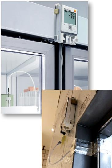
1. Determine location for the wall bracket and data logger on the outside of the refrigerator/freezer. Cable must be able to reach inside unit. Refer to the length of cable.
