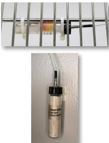
1. Take the probe (connected to the data logger) and poke it through the top part of the buffer bottle. Note: Recommended to have the probe 90% inside the buffer bottle and 10% outside the bottle.
