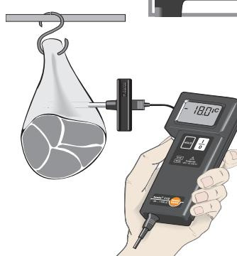
Disconnect the connection lead before removing the probe.
