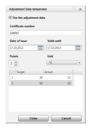
Once the calibration data has been entered, this is stored in the probe permanently. The probe takes deviations into account automatically during measurement, thereby generating a zero-error display.
