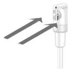
The correct measuring value is determined by rotating the probe slightly in both directions until the maximum value is displayed.
