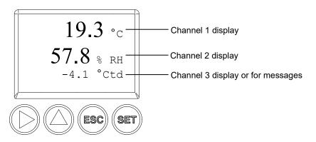
Four keys enable the user to navigate/scroll through the menus and enter/amend values and settings:
