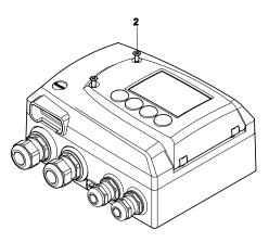
2 Close the service flap and tighten screws (2).
