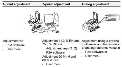
Either the 1-point adjustment or the 2-point adjustment is suitable for adjusting the sensor signal - digital signal chain.
