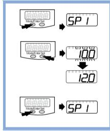
Press the **Mode/Enter** button until the **required parameter** appears on the display.
