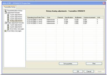
Selection of adjustment histories: 1-point adjustments / 2-point adjustments / Analog adjustments / n-point adjustments.
