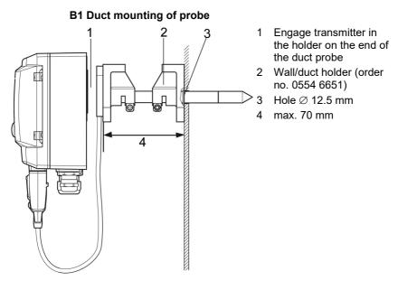
Only atmospheric processes up to approx. 1000 hPa positive pressure. Alternatively, the single-hole duct holder (order no. 0554 1793) can also be used.
