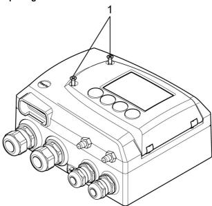
1. Loosen screw connection (1) of service flap and open the flap.
