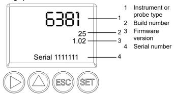
The serial numbers of the transmitter and probe can be read off.
