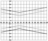
Grey line: System error 6381 + probe, electronics 25 °C/+77 °F Black line: System error 6381 + probe, electronics –25 to 70 °C/-13 to 158° F
