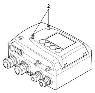
2. Close the service flap and tighten screws (2).
