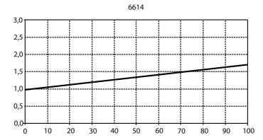
Temperature error as a factor of process temperature and temperature of electronics
