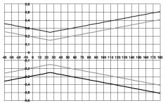
Grey line: System error 6381 + probe, electronics 25 °C/+77 °F Black line: System error 6381 + probe, electronics –25 to 70 °C/-13 to 158° F
