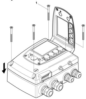
1. Place upper part of instrument on top of lower part (see arrow) and fix in place with housing screws (1).
