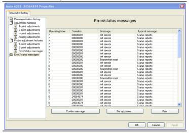
The table is shown only for error and status messages that were generated in the transmitter and were transferred and saved there via the connection to the P2A software.
