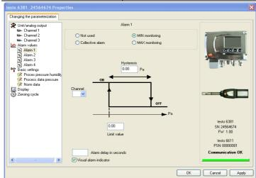
The graphic display in the centre of the screen refers to the relay wiring as a NO contact (ON).
