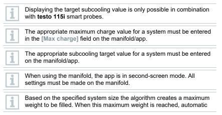
filling is paused and must be restarted. This prevents overfilling or incorrect filling.
