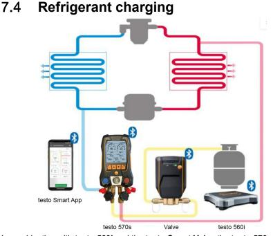
In combination with **testo 560i** and the **testo Smart Valve** the **testo 570s** offers multiple functions to charge refrigerant systems.
