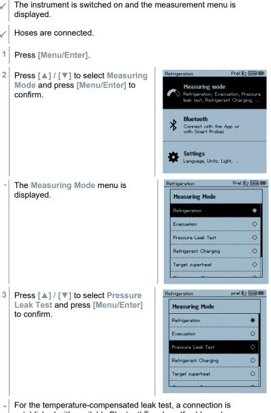
For the temperature-compensated leak test, a connection is established with available Bluetooth<sup>®</sup> probes. If cable probes are connected to the instrument, they are prioritized for the compensation. Please note that only air probes are ideal for temperaturecompensated leakage testing.
