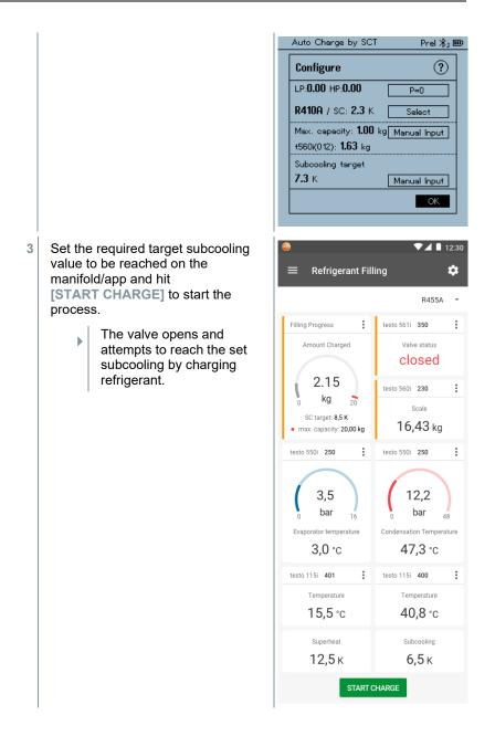
Added refrigerant is displayed in g/kg increments on the manifold/app.
