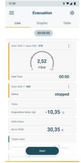
The measurement is running, the vacuum holding test has not yet started.
