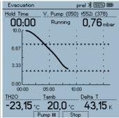
When the target values are reached, the evacuation and therefore also the pump are stopped automatically. The vacuum hold test begins.
