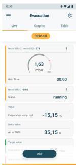
When the target values are reached, the evacuation and therefore also the pump are stopped automatically. The vacuum hold test begins.
