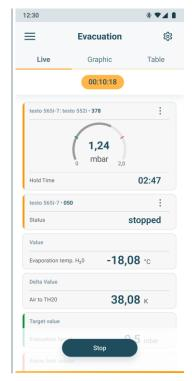
If the Auto Re-Start function has been activated, evacuation is restarted in order to restart the vacuum hold test once the target value has been reached.
