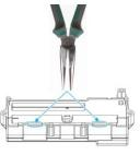
Remove the battery from the housing.
