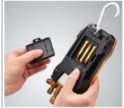
3 Loosen the 6 marked screws and remove the back of the device.
