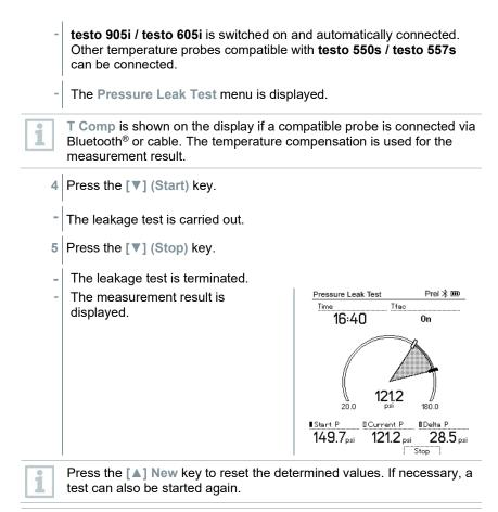
The measurement result can be displayed graphically on the manifold as well as in the app.
