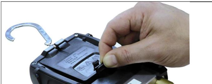
1. Fold out the suspension device, loosen the clip and remove the cover of the battery compartment.
