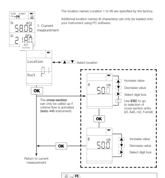
From now on all measured data which is saved or printed is
