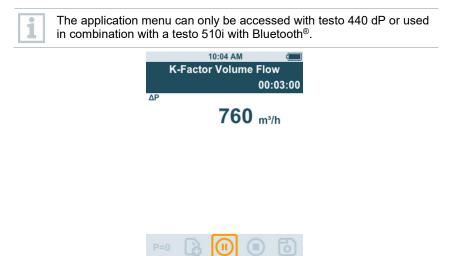
This process for determining volume flow can always be used when there are appropriate specifications available from the component manufacturer. In line with these specifications, the differential pressure is measured at a position specified by the manufacturer or supplier. The volume flow is determined from the differential pressure via a component-specific K-factor using the following mathematical equation:
