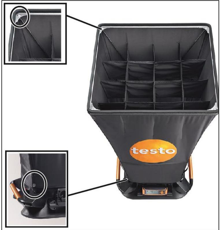
1. Pull the lower end of the hood over the measurement base.
