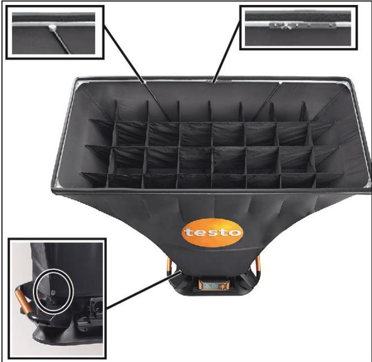
1. Install the aluminium frame and stretch the fabric hood over the framework, so that the elastic band lies in the recess of the frame. Make sure that the elastic band fits correctly, especially at the corners.
