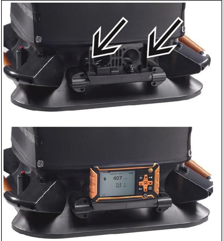
1. Push the testo 420 completely into the instrument holder, pay attention to the catch on the right-hand and left-hand side in the bracket.
