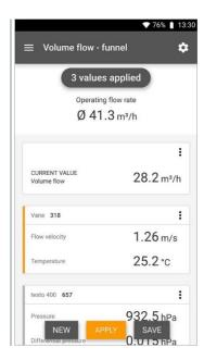
6 Apply: the current reading is applied.
