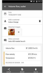
The calculated result of the measurement is displayed under the Customer data, Images and Comments.
