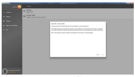
As soon as the testo 400 is connected via a USB cable to a computer, Connected to testo 400 – Synchronizing is displayed at bottom left. A message about data transfer is displayed. Confirm by pressing OK to transfer all customer and measurement data from the testo 400 to the software. The testo 400 memory is then empty. Depending on requirements, customer and
