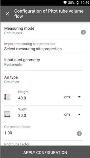
Configuration of Pitot tube volume flow
