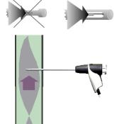
The flue gas must be able to flow freely past the thermocouple.
