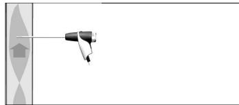
The tip of the probe must be in the core current of the flue gas flow.
