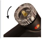
Remove particle filter (1) and store it 2 to reinsert it after the measurement.
