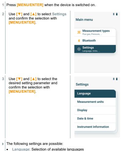
Measurement units: Changing temperature unit and pressure unit
