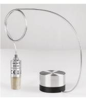
3 Bend the probe shaft so that the freeze-drying probe holder is in full contact with the plate.
