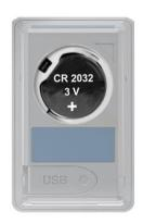
7 Place battery compartment cover on the data logger and close it by turning it to the right.
