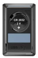
7 Place battery compartment cover on the data logger and close it by turning it to the right.
