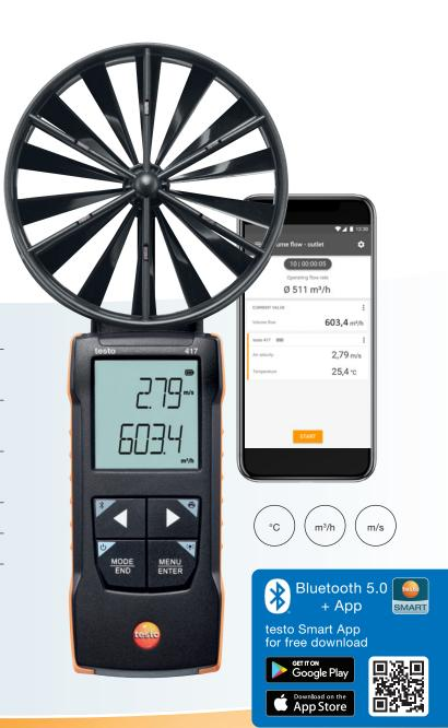
The compact vane anemometer testo 417 was developed to make it as easy as possible for you to take measurements on air inlets and outlets of **air conditioning and ventilation systems**. The integrated 100 mm vane quickly ensures precise results. Time and point average values as well as the volume flow are automatically calculated in the instrument and shown on the display.
