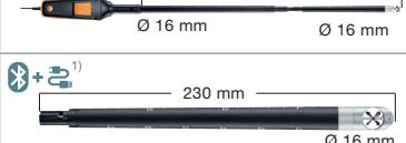
230 mm<br>Ø 16 mm                   | 0 to 50 m/s<br>-10 to +70 °C                                   | ±(0.2 m/s + 1% of m.v.)<br>(0.6 to 40 m/s)<br>±(0.2 m/s + 2% of m.v.)<br>(40.1 to 50 m/s)<br>±1.8 °C                                                                                                                                                                                                                                | 0.1 m/s<br>0.1 °C                        | 0635 9570 |
