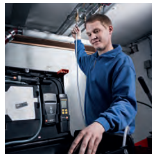
Drinking and waste water test with high-pressure probe up to 25 bar
