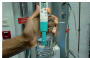
Ideally suitable for monitoring heating system water according to VDI 2035.
