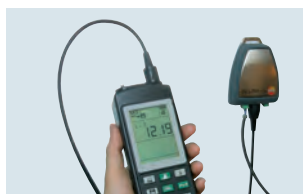
Inspection of transmitters with 4 to 20 mA interface
