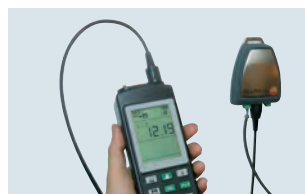
Inspection of transmitters with 4 to 20 mA interface
